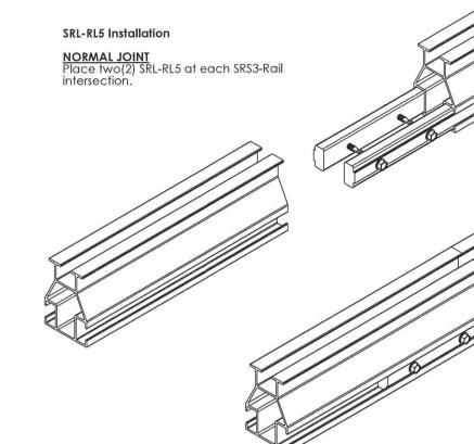
THERMAL EXPENSION JOINT Once every 40' (once every two rails), leave a 12mm gap between rails and screws (2 screws on each side, 4 total) the SRL-RL5 only to one of the SRS3-Rail.
