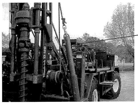
Hammering device in stand-by position.
