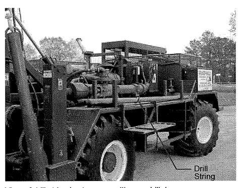
View of drill string in storage position on drill rig.
