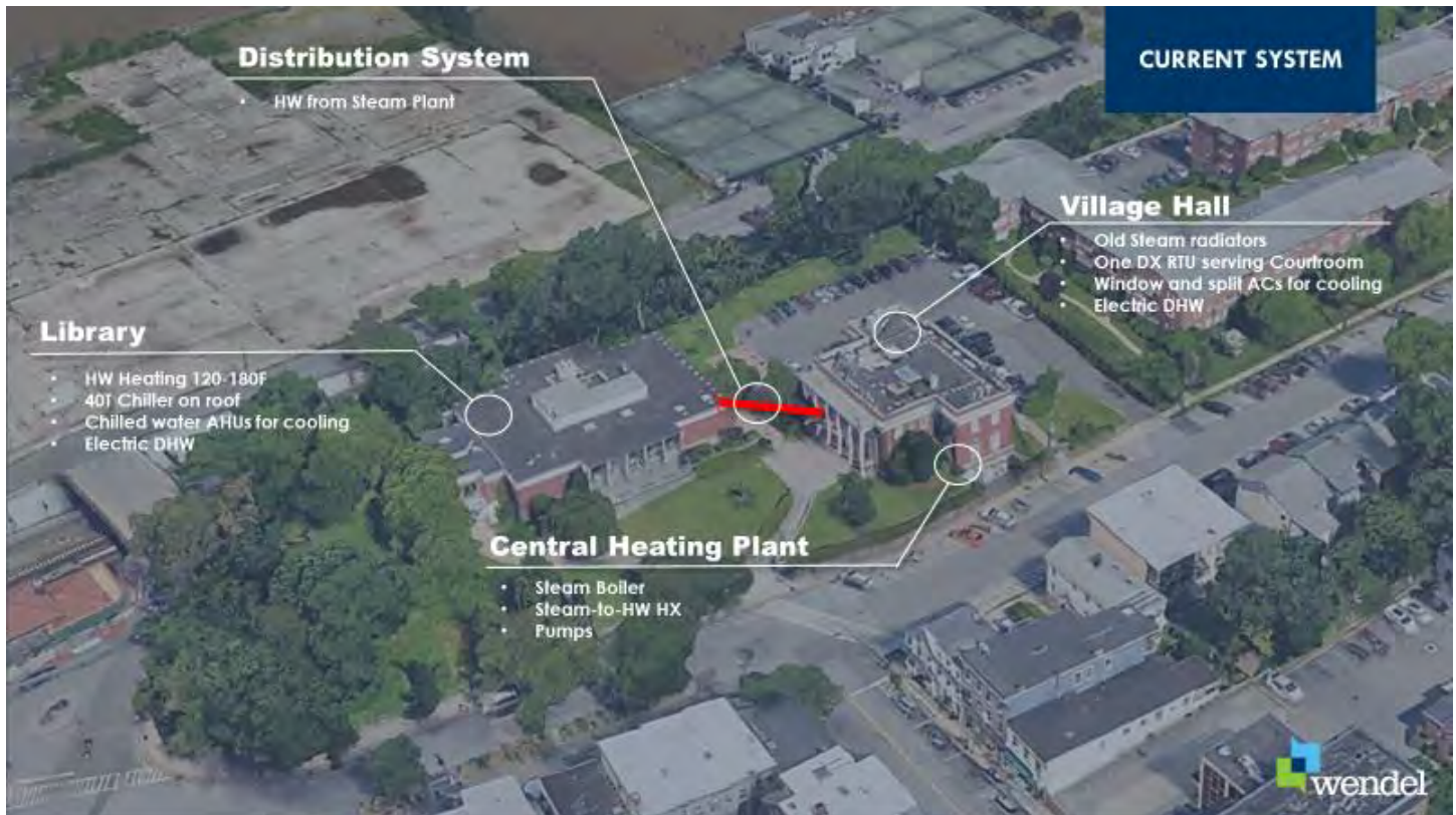
Figure 1. A summary of the existing heating and cooling distribution systems at the Village Hall and Library
