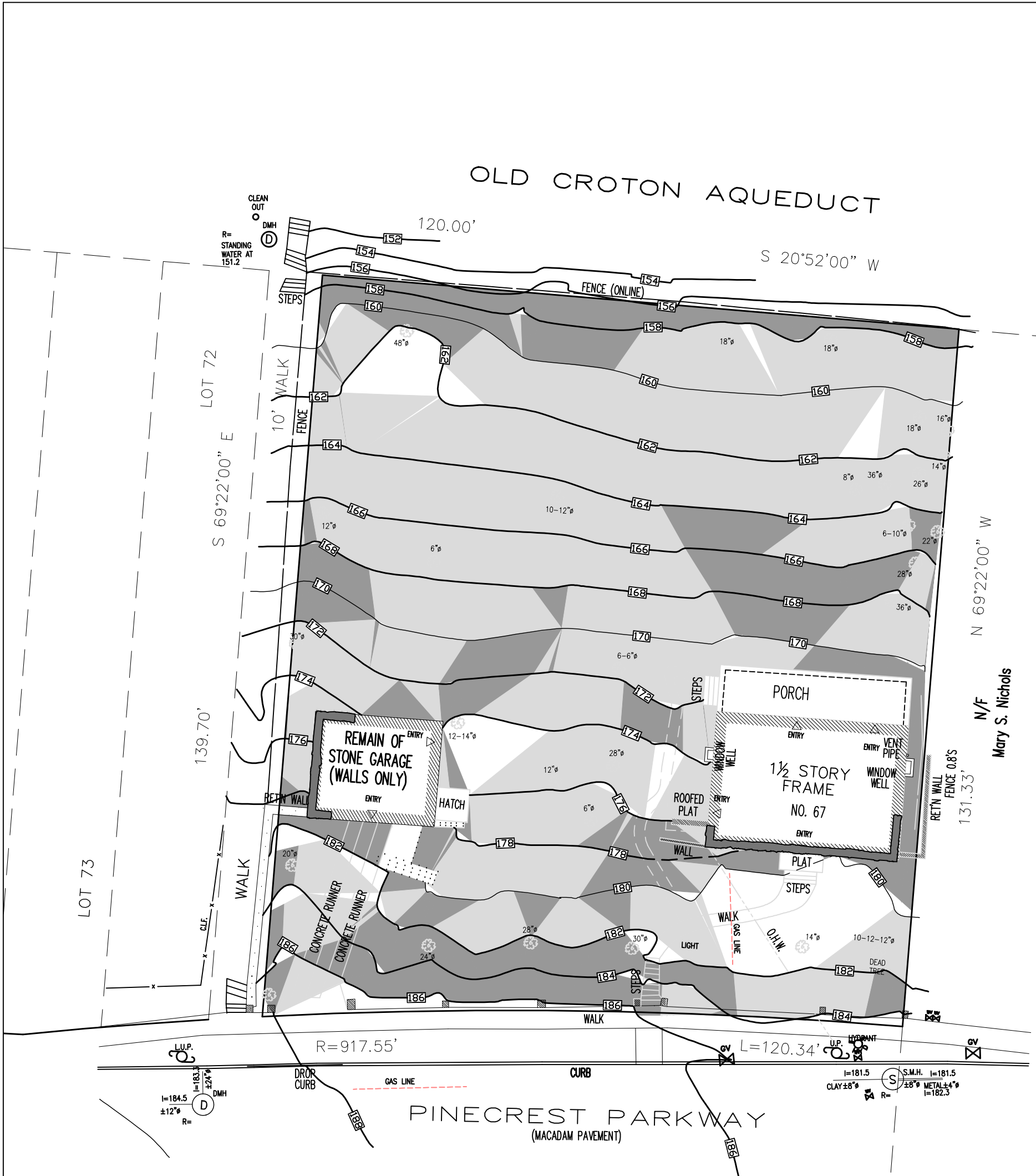
LAYOUT A: EXISTING CONDITION SLOPE ANALYSIS SCALE: 1" = 20'
