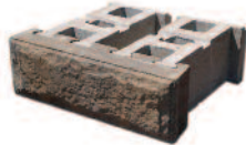
824 facing unit w/LAU Approx. 0.75 blk/ft 2 (8 blk/m 2 ) 8 in. H x 23 in. D x 24 in. L (200 mm H x 585 mm D x 600 mm L) 185 lbs (85 kg)
