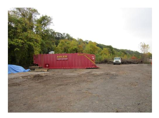
Photo 2: Frac tank and water truck
