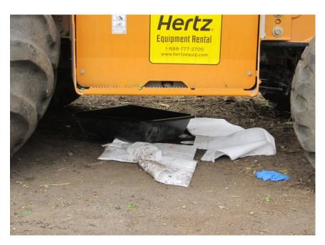
Photo 2: Hydraulic line leak on Backhoe
