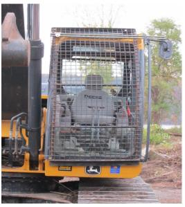
Photo 1: Shield for excavator
